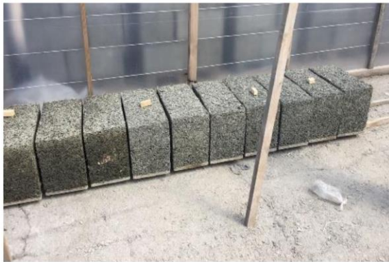
Figure 1 – Ready-made wood-cement composite blocks
